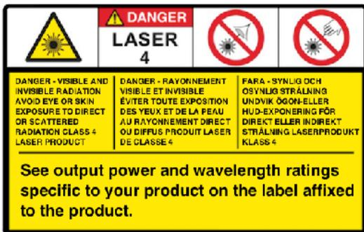
**Warning:** This product contains Class 4 laser sources. Avoid eye and skin exposure to direct or scattered visible and invisible laser radiation.
